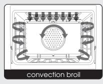
**\*Note:** This function uses a high-speed convection fan for optimum cooking performance. Some noise may be noticed from this high fan speed. This is normal.
